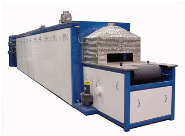
Figure 7. Straight through continuous steam treater
