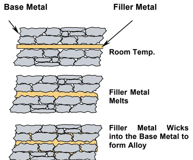
Figure 2. Brazing Schematic
