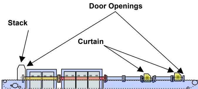
Figure 8. Stainless Steel Brazing Furnace Schematic
