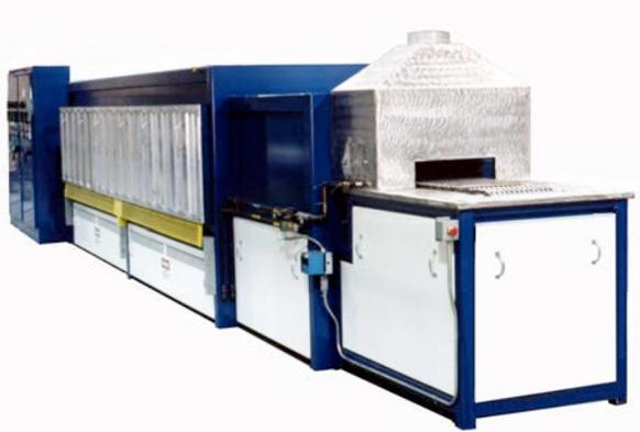
Figure 1. Controlled Atmosphere Brazing Furnace.
