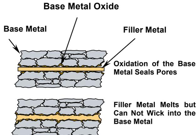
Figure 4. Effect of Oxidation on Brazing. The level of cleanliness is much more important for stainless steel components than brazing steel components. The Chromium in the stainless steel forms a much more stable oxide at a much lower Oxygen level than Iron.
