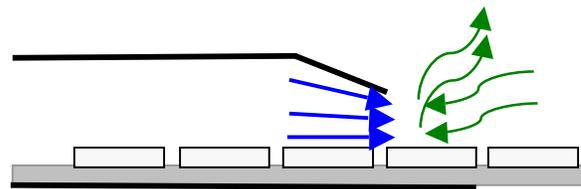
Figure 9. Flow Exiting the Door Prevents Air Infiltration.
