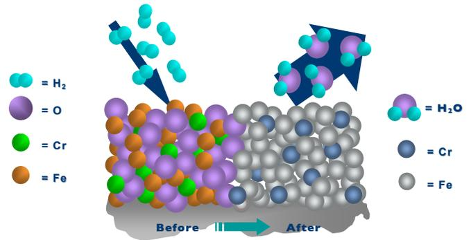
Figure 6. Oxide Reduction Mechanism
