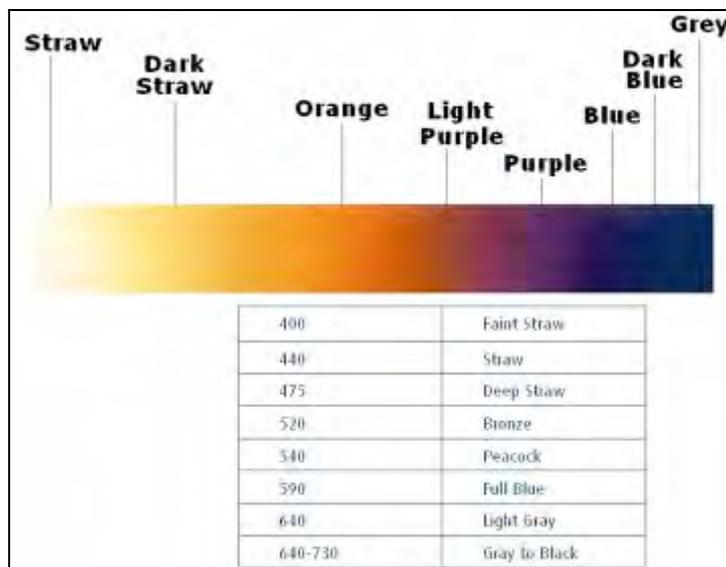
Figure – 6 Oxidation Colours – temperature is in Degrees Celsius
