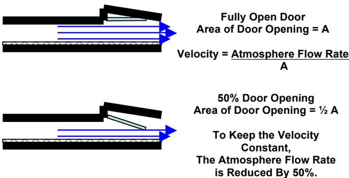
Figure 3. Effect of Door Position on Atmosphere Flow Rate
