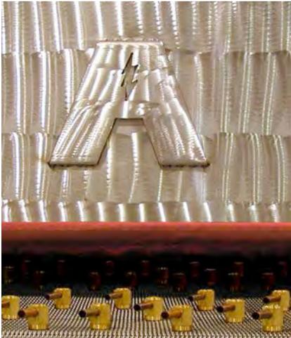
Figure 1. Parts Entering a Continuous Brazing Furnace.
